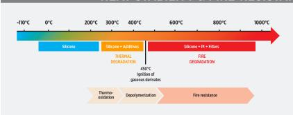
During the burning of silicone rubbers, some volatile and cyclic molecules are produced with self-ignition near 450°C and are transformed into inert silica, H2O, SiC and CO2. By consequence, low smokes emissions are nontoxic, noncorrosive and halogen free. This behavior allows a safe and quick evacuation of people during the event of fire.
